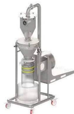
Delfin SEP.DC-020 cyclone separator with BIBO H14 filter unit for OEB 4 containment
