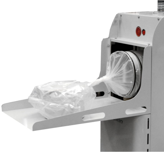
BIBO filter replacement on the Delfin SEP.DC-020
