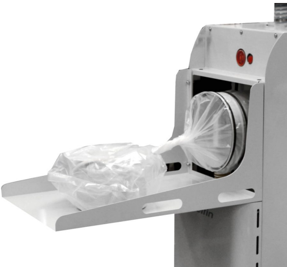
BIBO filter replacement on Delfin PHARMA 40.40 DC
