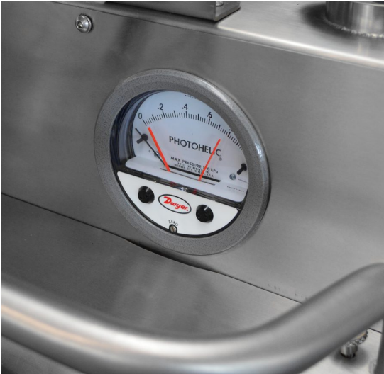
Photohelic filter indicator for Delfin PHARMA 40.40 DC
