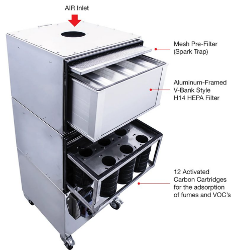
CD-595 EX HEPA VOC three-stage filtration system
