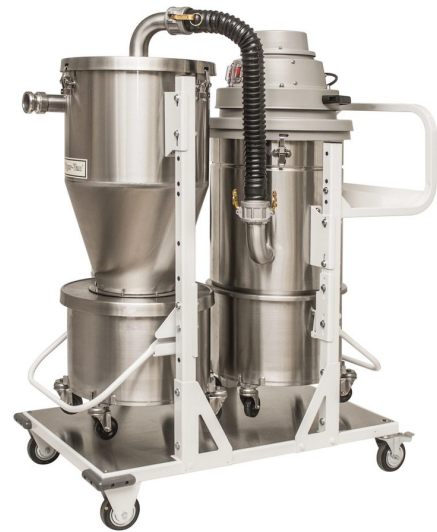
Tiger-Vac C-10 EX DT (PRS-HEC) – ATEX Zone 20 internal IECEx powder recovery system
