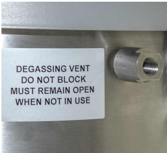
Degassing vent on ATEX-10A — must remain open when not in use
